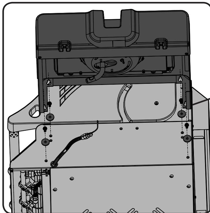
Fit orifice into burner tube and secure with hose retainer clip supplied. Attach the wire to the side burner electrode.
