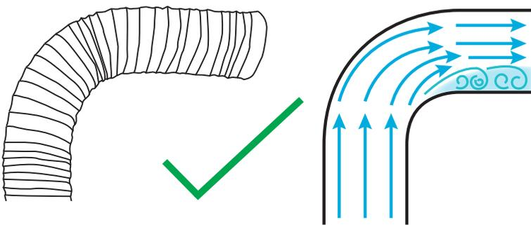
2. Sweeping curves and taut ducting reduces resistance and turbulence. The airflow and extraction will be more efficient and stronger.
