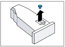
2. Insert the stopper on the underside.
